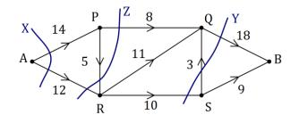
(a) Cut *X* passes through edges *AP* and *AR*, and cut *Y* passes through edges *RS*, *SQ* and *QB*. Show these cuts on the network and state their capacities. (2 marks)
